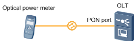
Figure 1-45 Measuring the Transmit Optical Power of an OLT PON Port
