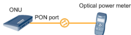
Figure 1-47 Measuring the transmit optical power of an ONU PON port
