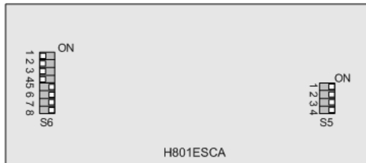
Figure 1-2 Layout of the DIP switches (in default settings) on the H801ESCA board
